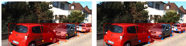
Fig. 2. Comparison between the 3D BBox's bottom vertices (orange dots) and the wheel pixels (blue dots). Obviously, the wheel pixels have stronger semantic information than the bottom vertices.
