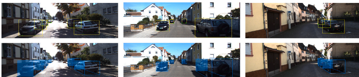
Fig. 10. The 2D BBox, wheel pixel and 3D BBox detection results. They are represented by yellow, green, and blue, respectively. Although some wheel pixels are blocked in the image, our model can still work well.
