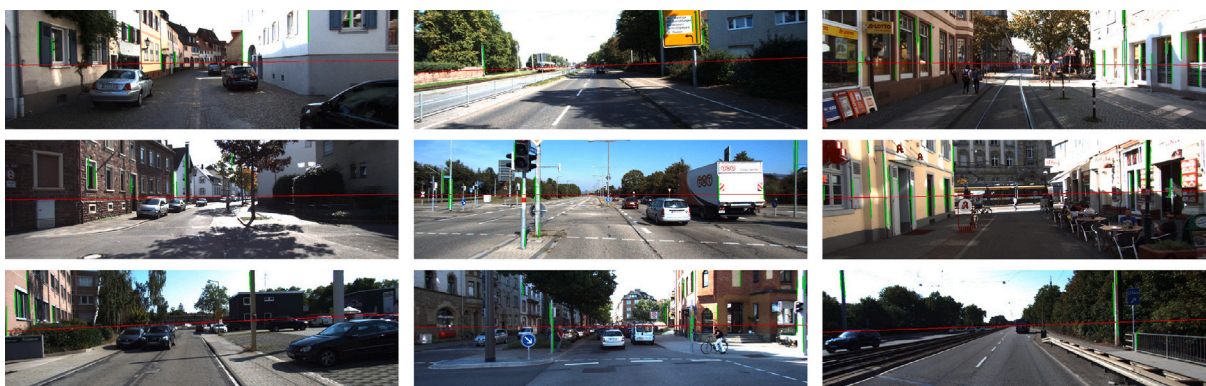
Fig. 9. Examples of the vertical edge and horizon line detection. The green lines are detected vertical edges, and the red lines represent the detected horizon lines in the image. The proposed vertical-edge-enhanced horizon line detection method can work effectively even if the horizon line is heavily occluded by obstacles.
