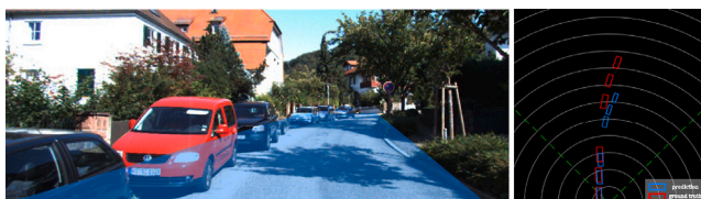
Fig. 3. The ground plane tilt problem in inverse projection. The blue plane is the preset fixed ground plane, neglecting the ground plane's tilt. From the bird's eye view (BEV), the inferred 3D BBox (blue box) using the fixed ground plane will gradually drift from the ground truth (red box).
