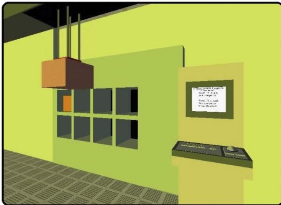
Fig. 1. The Virtual CVD Learning Platform (Koretsky et al., 2008). Figure shows loading of wafers into a CVD furnace within 3D graphical user interface.
