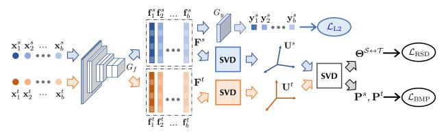
*Figure 3.* The architecture of our method. RSD is a novel distance to learn transferable representations for DAR problems. BMP is a novel regularizer to maintain geometrical structures of deep representations. They are end-to-end trainable by **differentiable SVD** in PyTorch.
