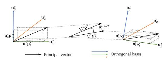
Figure 2. The calculation process of principal angles. Principal angle  $\theta_1^{S \leftrightarrow T}$  is the angle between principal vector  $\mathbf{U}^s \mathbf{p}_1^s$  and  $\mathbf{U}^t \mathbf{p}_1^t$ . Principal vector  $\mathbf{U}^s \mathbf{p}_1^s$  is the *weighted sum* of orthogonal bases  $\mathbf{U}^s$ , where  $\mathbf{p}_1^s$  is corresponding weight vector.
